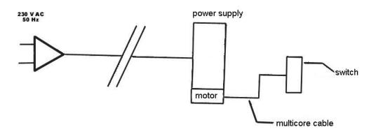
WARNING! Please note that the actuator/motor should be ran intermittently: max 2 minutes on/18 minutes off.
