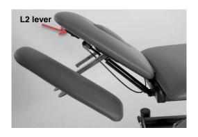
The headrest can be adjusted through a gas spring operated with a specific lever. In order to adjust the inclination, pull the lever (L2) and set the desired position; when the desired position has been reached, release the lever (L2).
