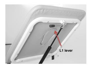
The headrest can be adjusted through a gas spring operated with a specific lever. In order to adjust the inclination, pull the lever (L1) and set the desired position; when the desired position has been reached, release the lever (L1).
