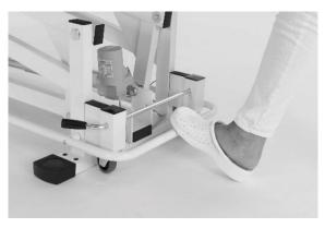
The height adjustment between 45 and 90 cm is operated by pushing or pulling the bar placed around the base of the couch.
